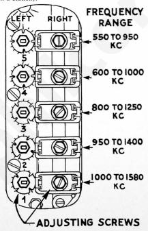
6—Hold the dial assembly against the edge of the instrument panel to complete the electrical connection and press the Automatic Station Selector button once. The dial will now rotate one position. The front slot is for the call letters of the station with the highest frequency in kilocycles.
